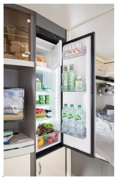
Spacious and convenient: the new 130-litre absorption refrigerator can be opened from both sides.
